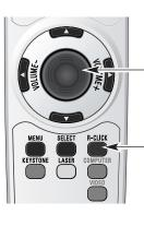
\_PRESENTATION POINTER button Move the pointer on the screen with this button.
