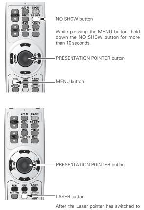
After the Laser pointer has switched to the Pointer, use the LASER button as the Pointer function ON-OFF switch. Press the LASER button toward the projector and see if it emits green light.
