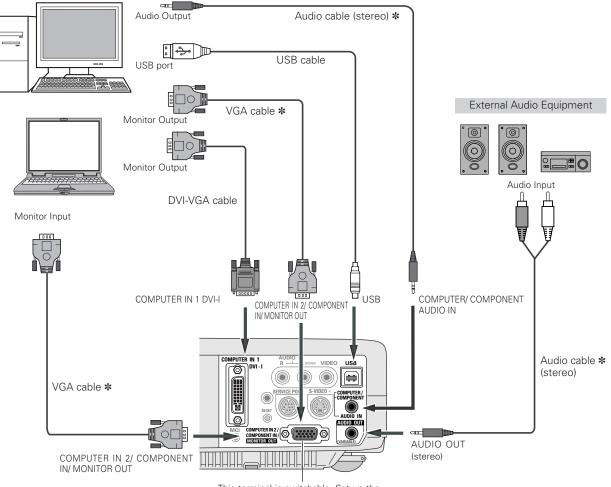
This terminal is switchable. Set up the terminal as either Computer input or Monitor output. (See Page 44.)
